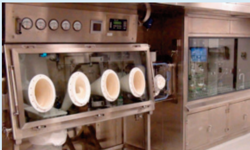
ADC isolator integrated with chemical hood via pass-through chamber: Photo courtesy of Howorth
