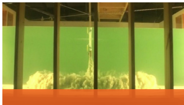
Figure 4: Physical modelling of open water slurry disposal
